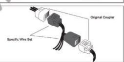
After fixing the specific Wire Set with coils, the remaining coupler of wire set to be connected with the Main Unit. Connection of the wire set with the Main Unit is as shown in the installation manual of DSPARK MAX Main Unit sold separately.
